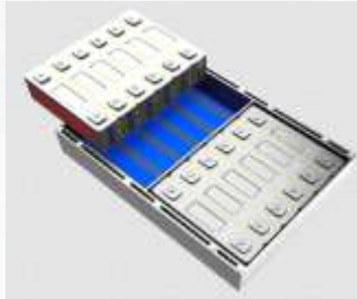
BATTERY CELLS IN A MODULE
