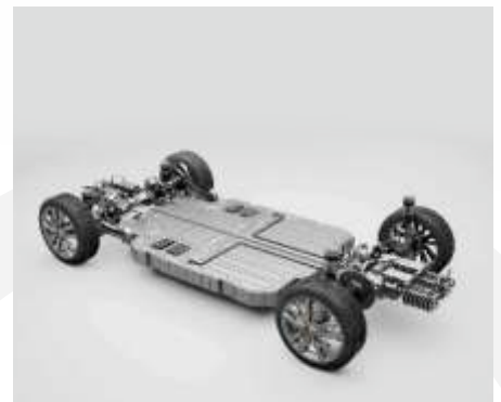
BATTERY AS PART OF THE CHASSIS
